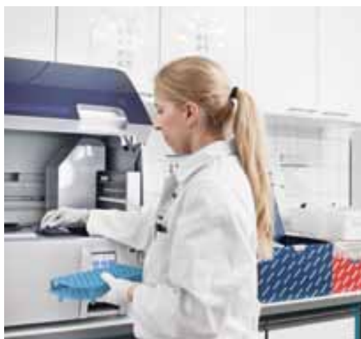
Scientist Andrea Düngelhoef loads samples into a QIAcube system for automated DNA extraction at the Center for Epidemiology near Bakum, Germany
