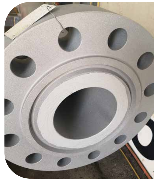
Pipe after inside coating.
