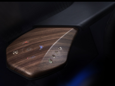
Centre console with fine wood panelling and integrated switch and lighting elements (smart surface)
